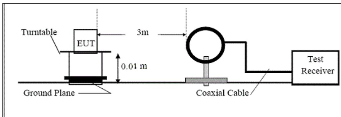
(B) For radiated emissions from 30MHz to 1000MHz
