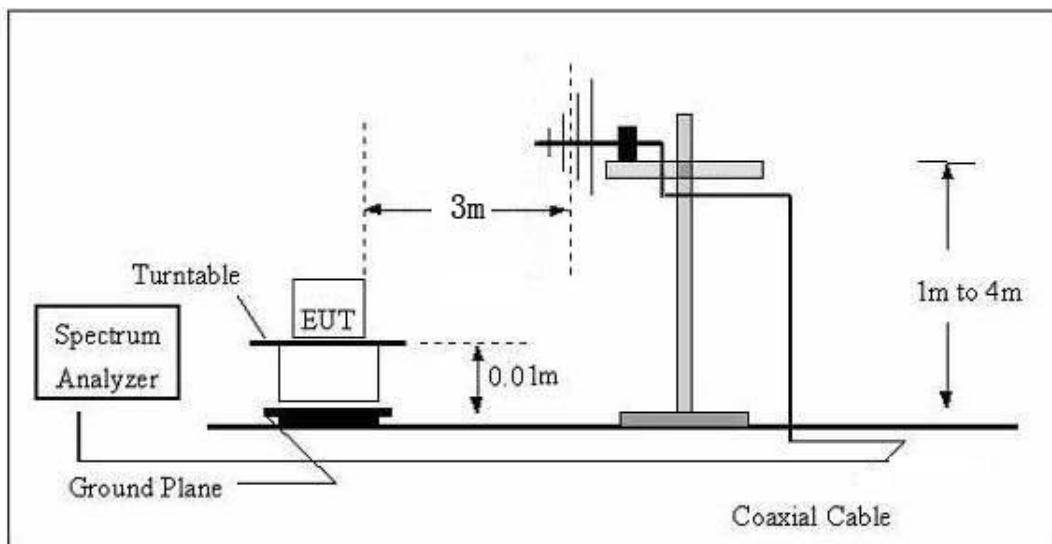
(C) For radiated emissions above 1000MHz
