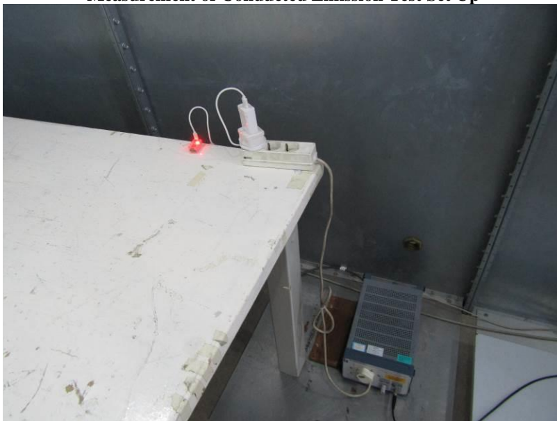
Measurement of Conducted Emission Test Set Up
