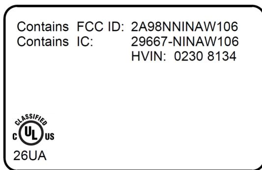
Labels are printed and glued on the backside of the remote control.
