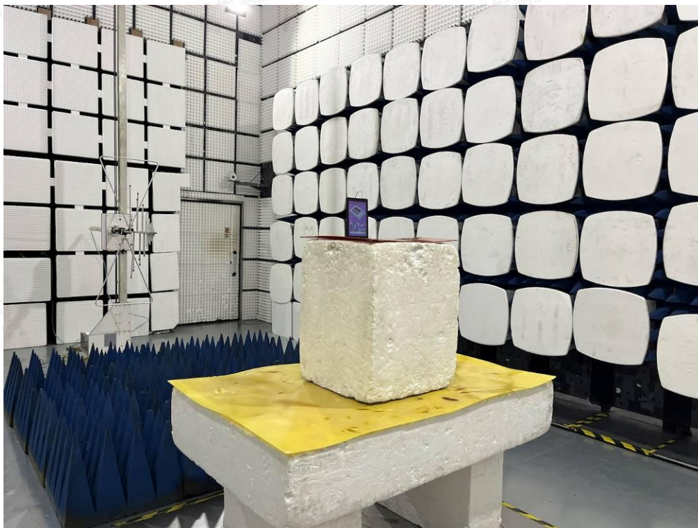
Radiated Emissions Measurement (Below 1GHz)
