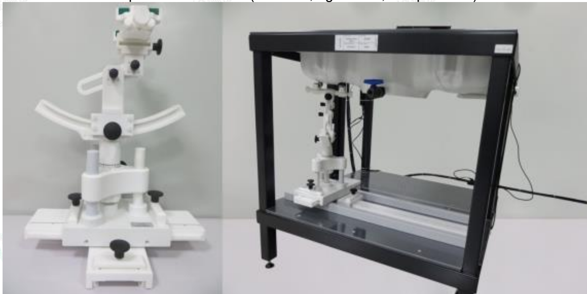
Device holder supplied by SATIMO
