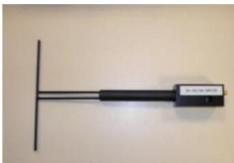
Figure 1 – Satimo COMOSAR Validation Dipole
