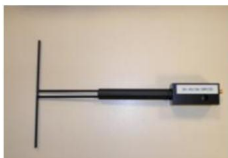
Figure 1 – Satimo COMOSAR Validation Dipole
