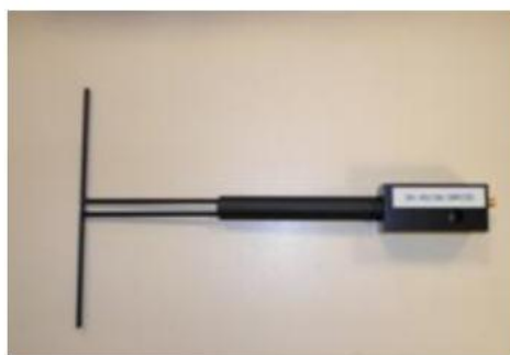
Figure 1 – Satimo COMOSAR Validation Dipole
