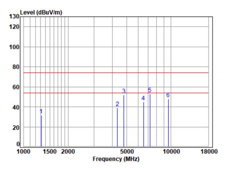
Site : chamber Condition: 3m VERTICAL : 02855HS/02856HS : 2402 TX RSE Mode : BLE-1M
