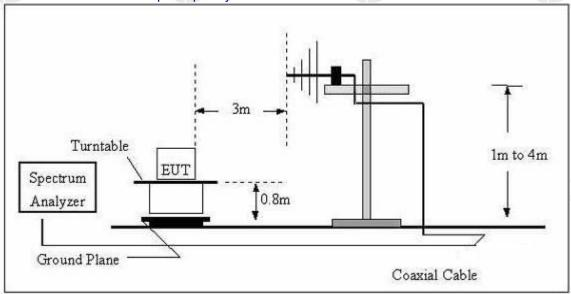
The radiated emission tests were performed in the 3 meters chamber test site, using the setup accordance with the ANSI C63.10-2013. The specification used was the FCC 15.209 and FCC 15.205 limits.
