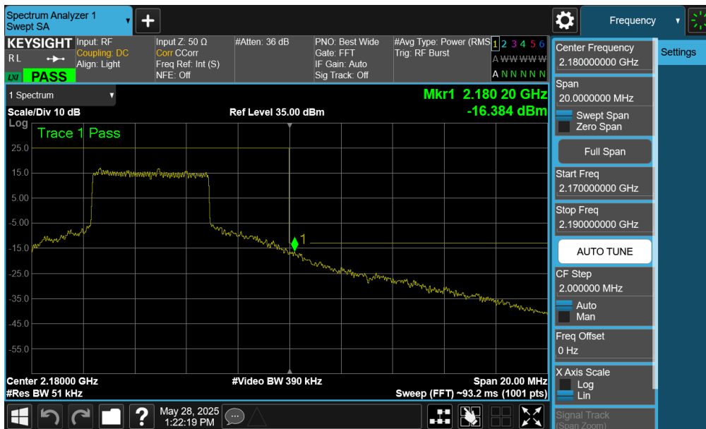
Plot 7-65. Upper Band Edge Plot (LTE Band 66 - 5MHz QPSK – Full RB)
