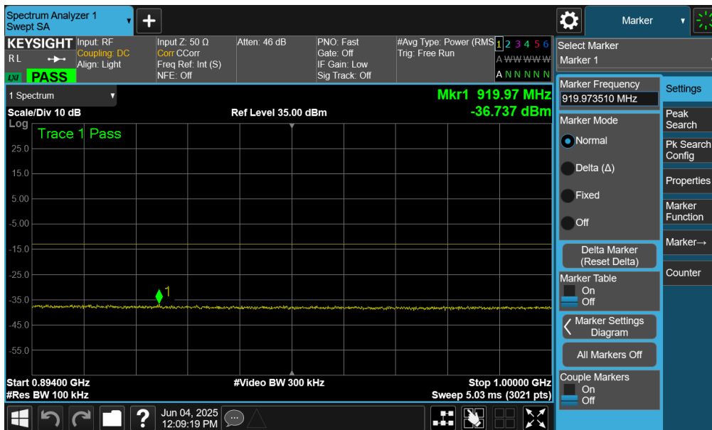
Plot 7-23. Conducted Spurious Plot (WCDMA Cell – Low Channel)
