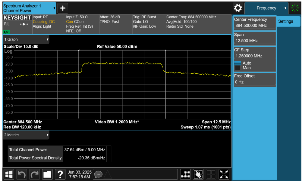
Plot 7-3. Conducted Power Output Data (LTE Band 26/5 – High Channel)
