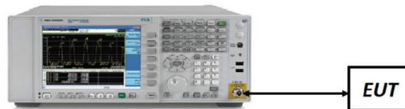
Figure 7-1. Test Instrument & Measurement Setup
