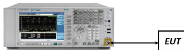
Figure 7-5. Test Instrument & Measurement Setup
