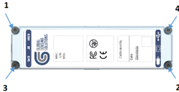
Figure 4 – Top Case Screw Removal Sequence
