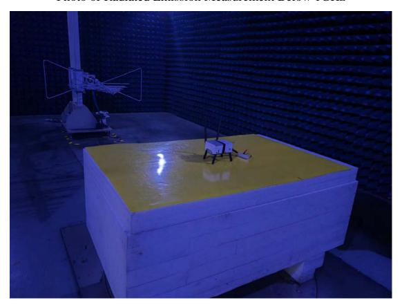
Photo of Radiated Emission Measurement Above 1GHz
