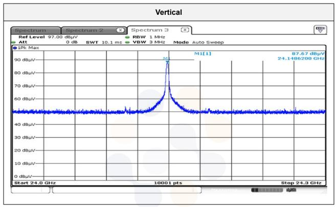
Note: The Average limit of fundamental is 107.96 dB $\mu$ V/m@3 m, and the maximum measure Peak level of fundamental is 90.41 dB $\mu$ V/m@3 m which is below 107.96 dB $\mu$ V/m@3 m, worst case of fundamental is recorded in this report.
