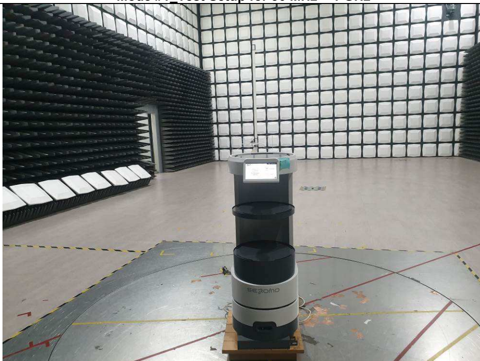
Mode #1 Test Setup for 30 MHz ~ 1 GHz
