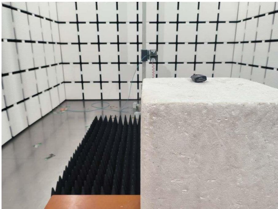
Radiated Emission Test View Above 1GHz
