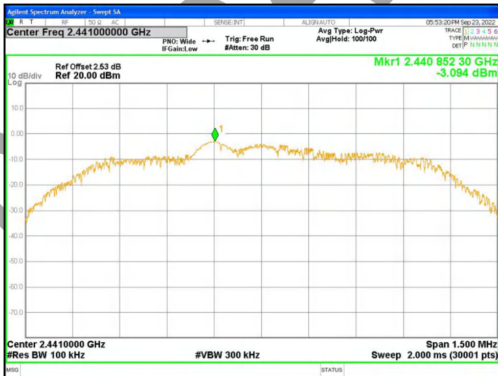
Tx. Spurious NVNT 2-DH1 2441MHz Ant1 Emission
