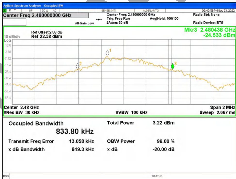
-20dB Bandwidth NVNT 2-DH1 2402MHz Ant1
