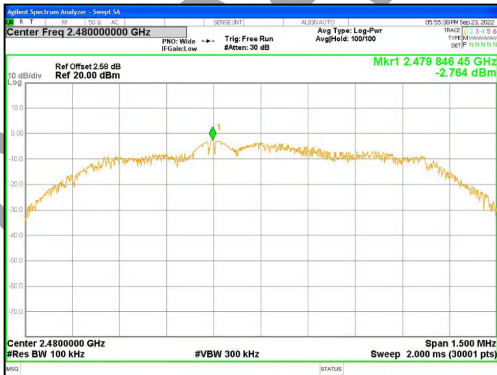
Tx. Spurious NVNT 2-DH1 2480MHz Ant1 Emission
