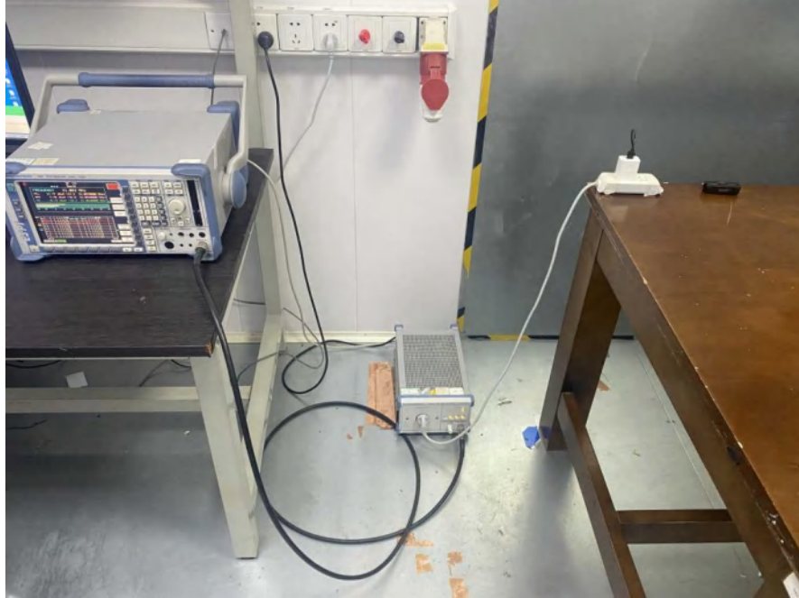
Conducted Emissions at AC Power Line (150kHz-30MHz)
