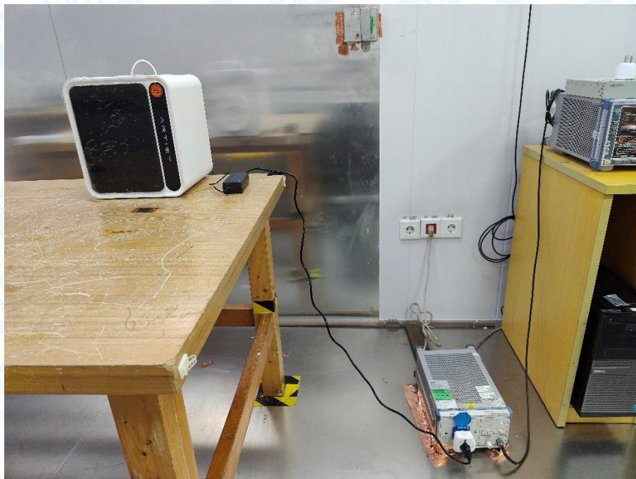
Photo of Setup for Conducted Emission
