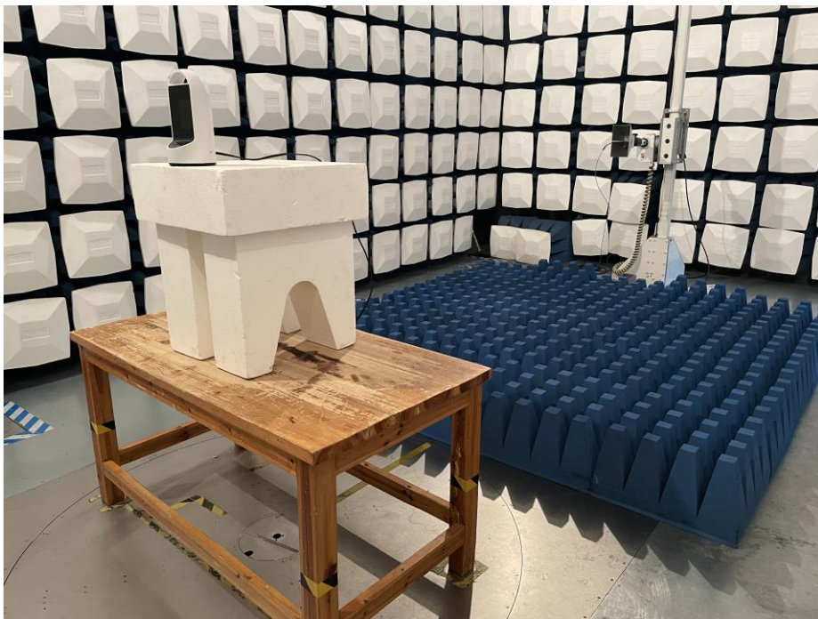
Test Setup For Radiated Emission (Above 1GHz)
