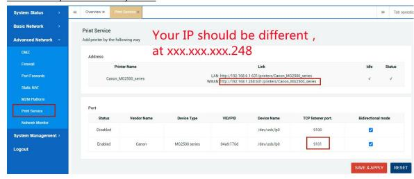
➤ If the Wi-Fi DHCP obtain IP address is not as of xxx.xxx.xx.248, Or this address is already occupied by another device. You have to manually set a static IP address for Print Server's WiFi WAN port as follows:
