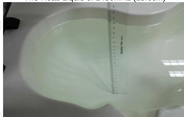
The Head Liquid of 1800MHz (15.2cm)
