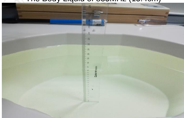
The Body Liquid of 1900MHz (16.4 cm)
