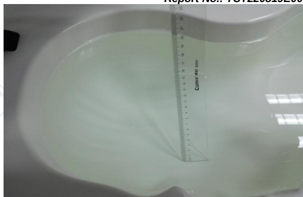
The Head Liquid of 2450MHz (15.6cm)
