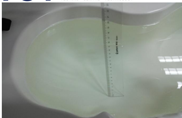
The Head Liquid of 1900MHz (15.5cm)
