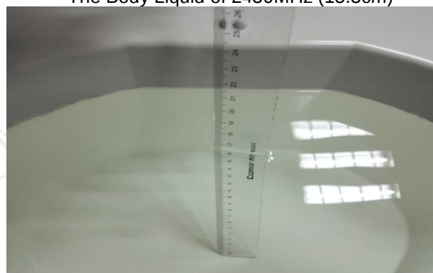
The Body Liquid of 5000-6000MHz (16.5cm)
