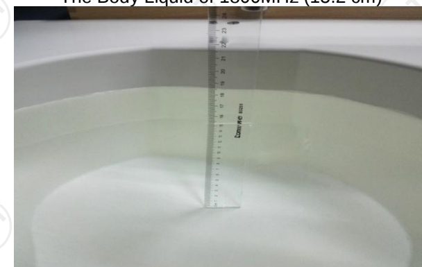
The Body Liquid of 2450MHz (15.3cm)
