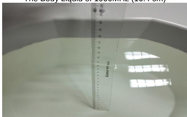
The Body Liquid of 2600MHz (16.5cm)
