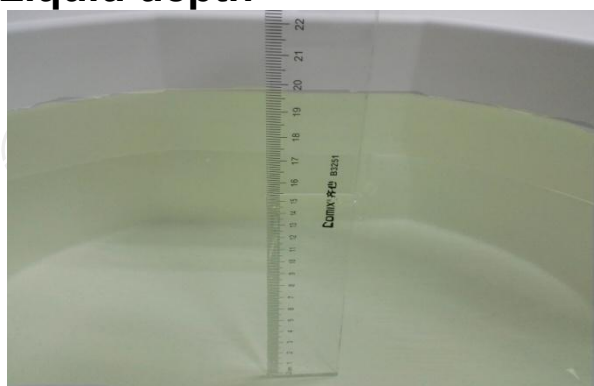
The Body Liquid of 835MHz (15.4cm)
