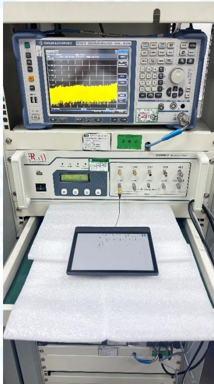
Photo of Setup for RF Conducted----GSM&WCDMA&LTE
