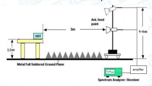
**Above 1GHz Test Setup**
