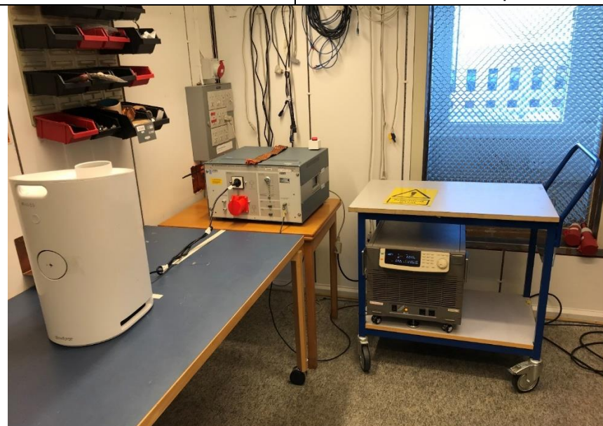
Photo 4.1.1 .....: Measurement of AC power-line conducted emission
