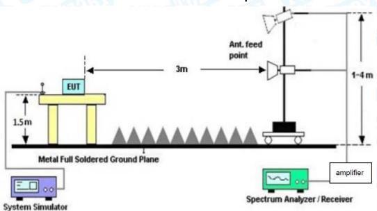
**Above 1GHz Test Setup**
