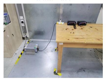
Radiated Emissions From 30MHz-1000MHz
