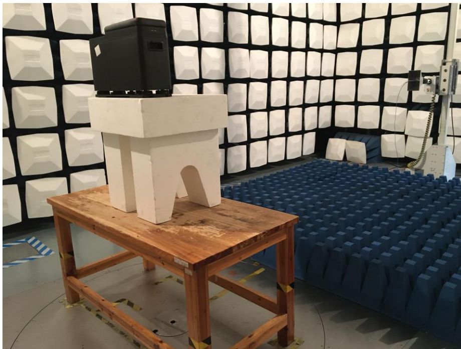
Test Setup For Radiated Emission (Above 1GHz)
