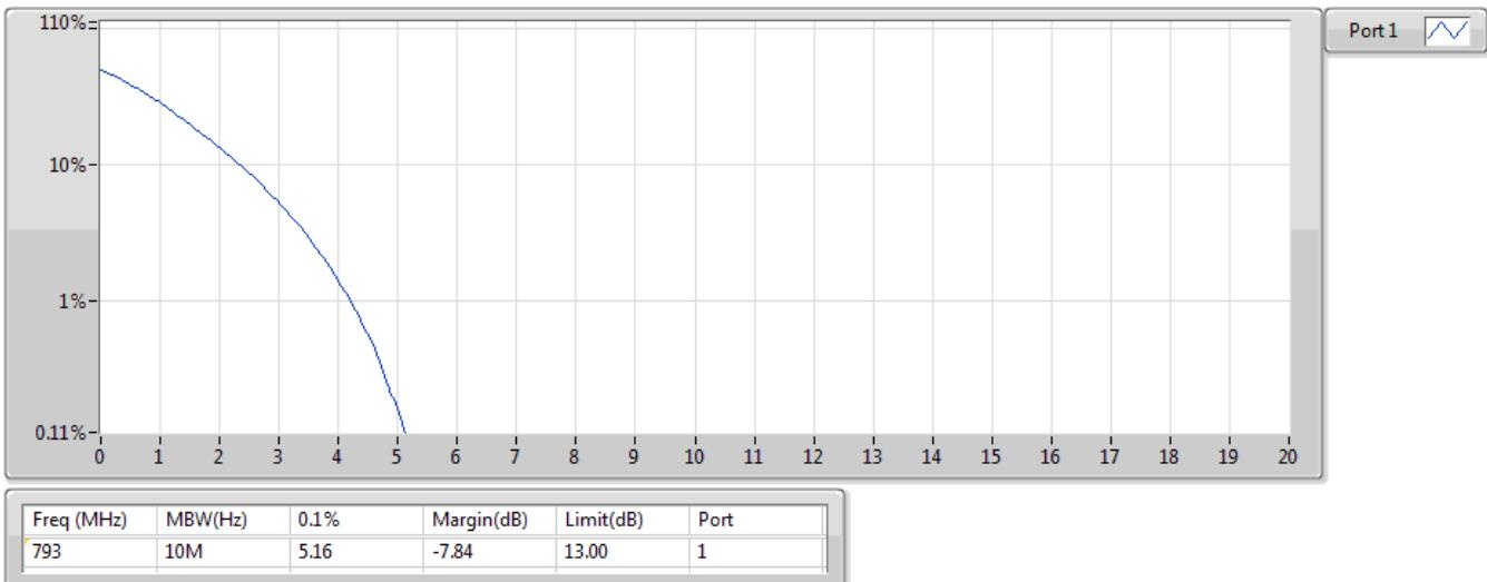
**Band 14\_LTE\_10MHz\_Nss1,16QAMCS\_1TX****PAPR****793MHz\_16QAM\_RB 50,#RB 0**
