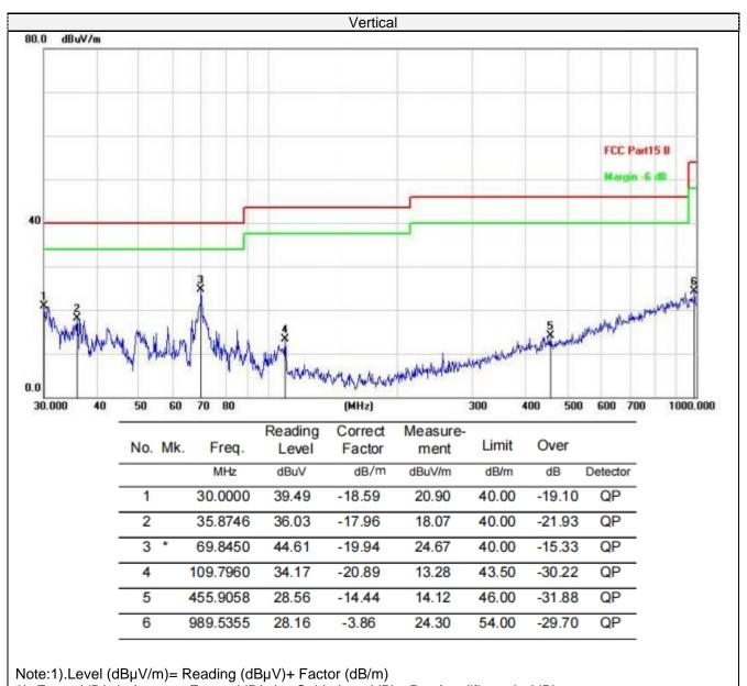
2). Factor(dB/m)=Antenna Factor (dB/m) + Cable loss (dB) - Pre Amplifier gain (dB)
