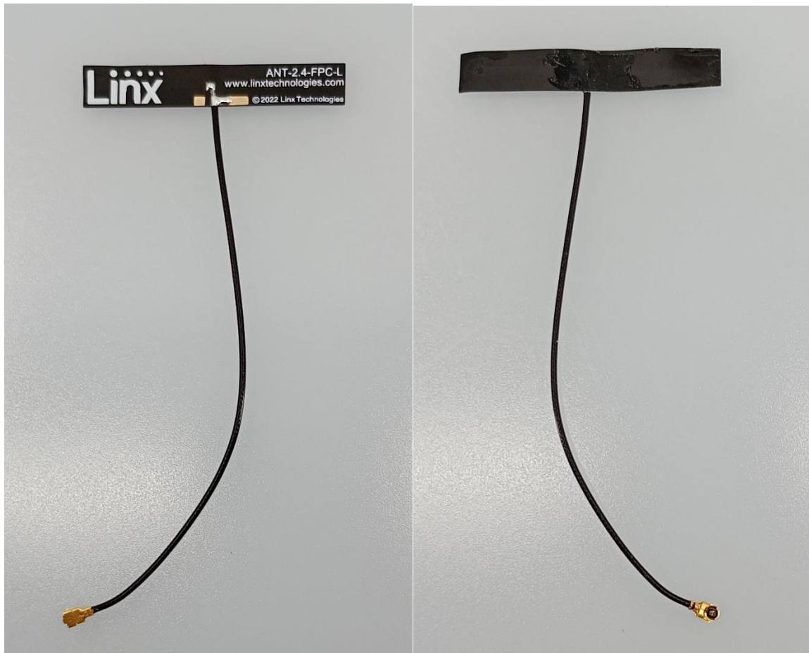
Figure 31 – 2.4GHz antenna (AP2 - ANT-2,4-FPC-LV100UF)
