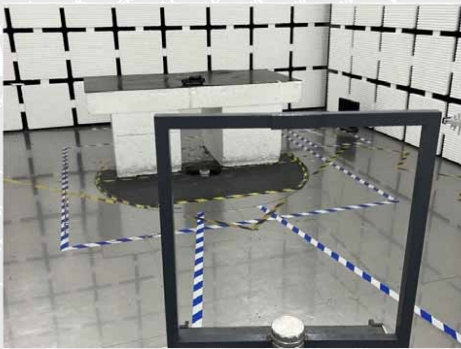
Radiation Emission Test Setup (Below 30MHz)
