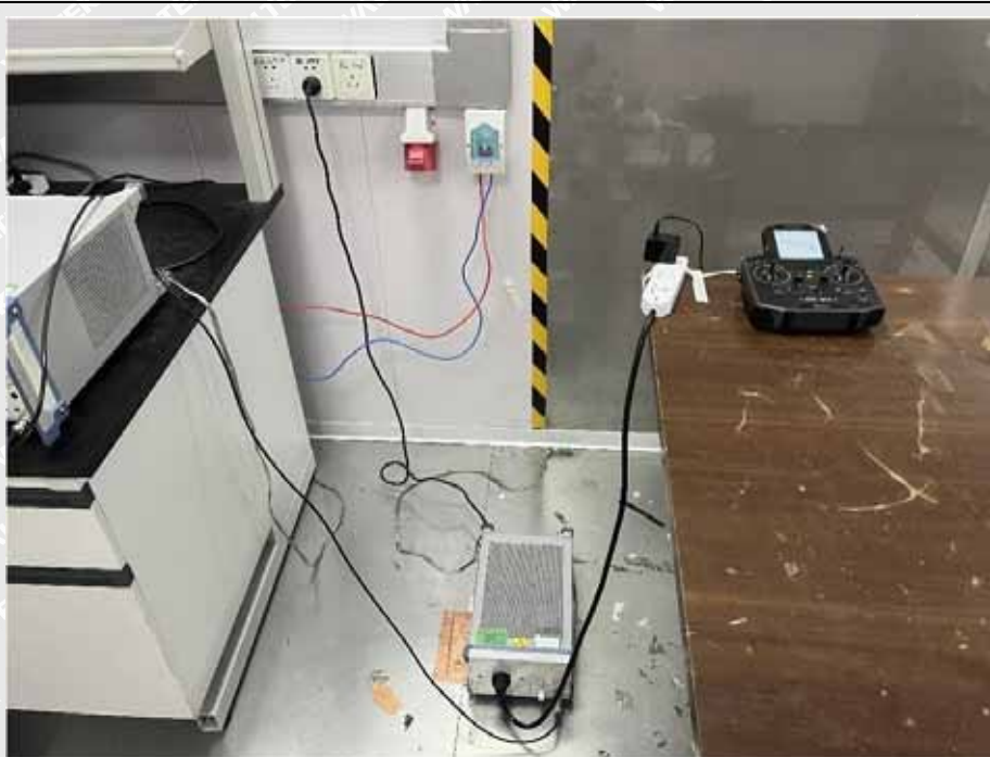
Conducted Emission Test Setup
