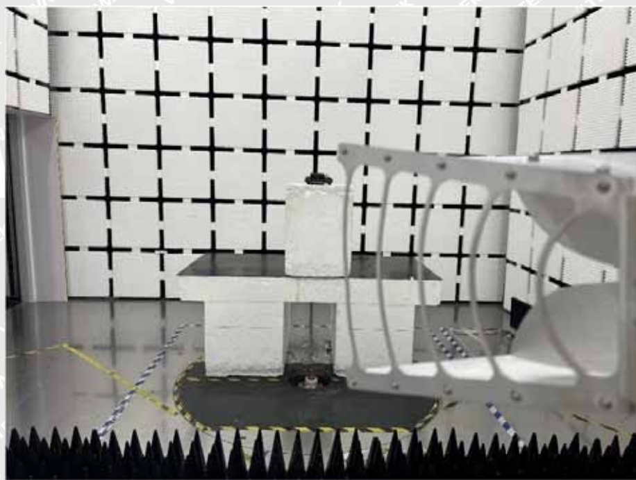
Radiation Emission Test Setup (1GHz to 18GHz)
