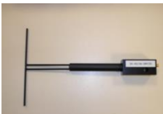
Figure 1 – MVG COMOSAR Validation Dipole
