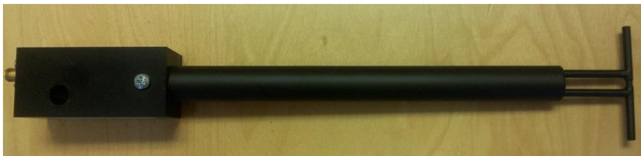
Figure 1 – MVG COMOSAR Validation Dipole
