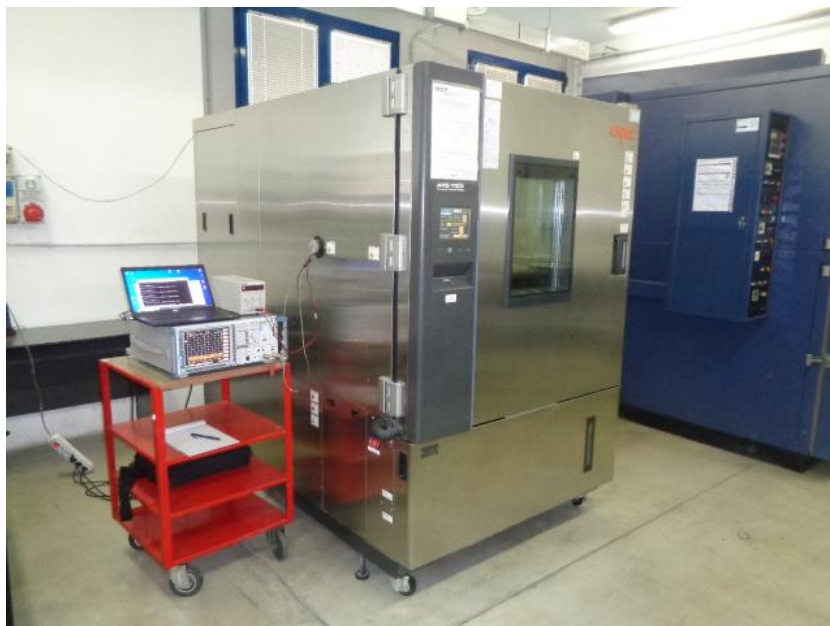
Figure 9.1-2: Antenna port testing set-up in climatic chamber
