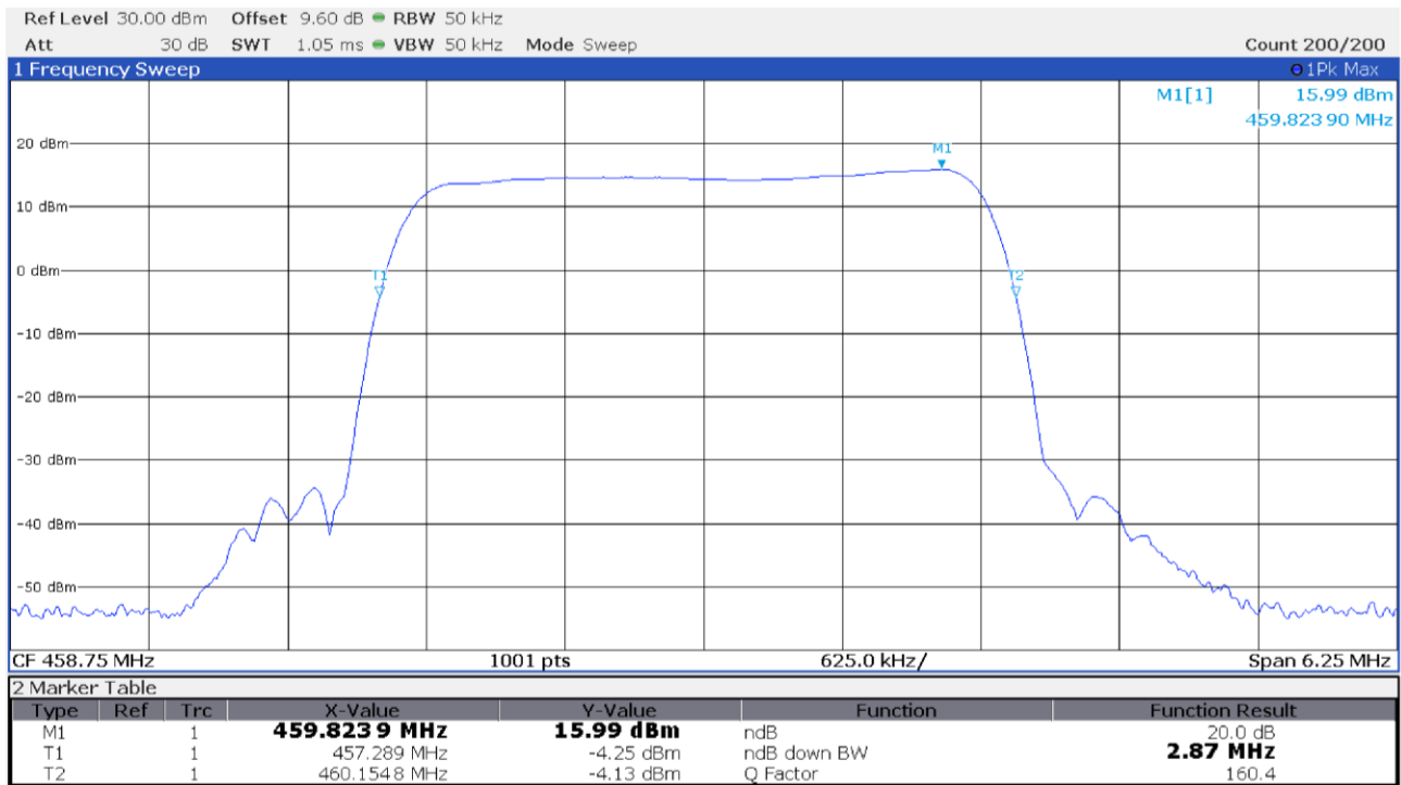
Figure 8.2-2: Out-of-band-rejection 20dB BW spectral plot for up link
