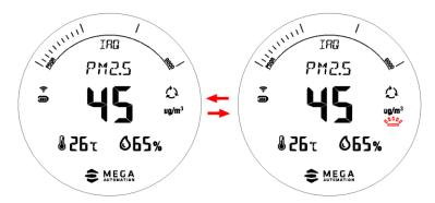
> Press [POWER/LIGHT] for a long time to switch on and OFF, and the shutdown will show off. Shut down after 1 second, shutdown interface diagram
