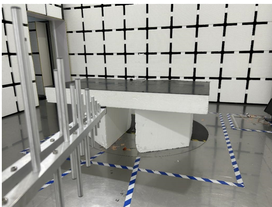
Radiation Emission Test Setup (30MHz to 1GHz)
