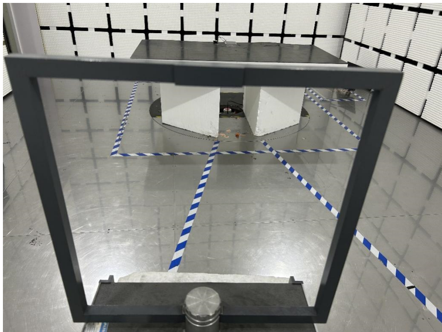
Radiation Emission Test Setup (Below 30MHz)
