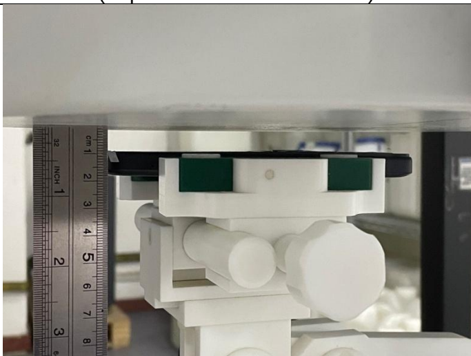
Front Side (Separation distance of 10mm)
