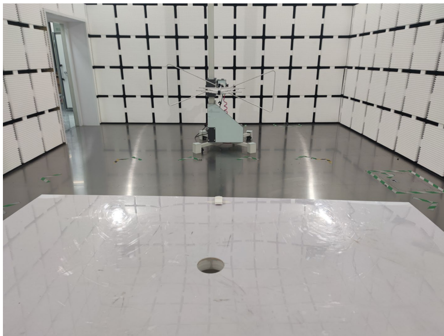
DTS Radiated Emission
