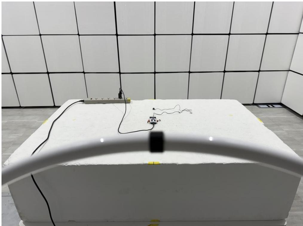
**Radiated emissions test photos****30 MHz to 1 GHz**
