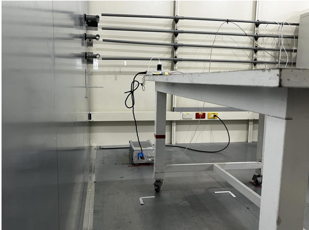
**Radiated emissions test photos****9 KHZ to 30 MHZ**
