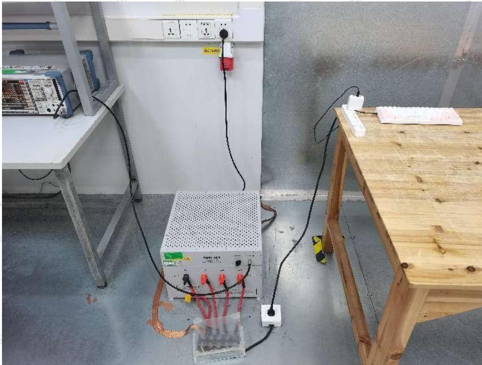
Photo of Conducted Emission Measurement
