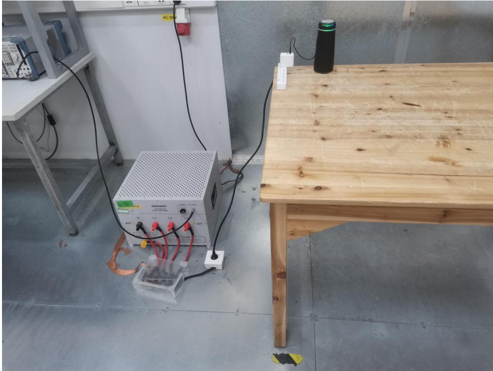
Photo of Conducted Emission Measurement
