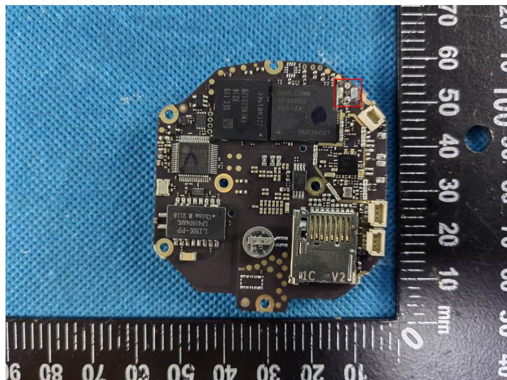
Inside the red square is the soldering point of the coaxial cable between the antenna connector and the mainboard.
