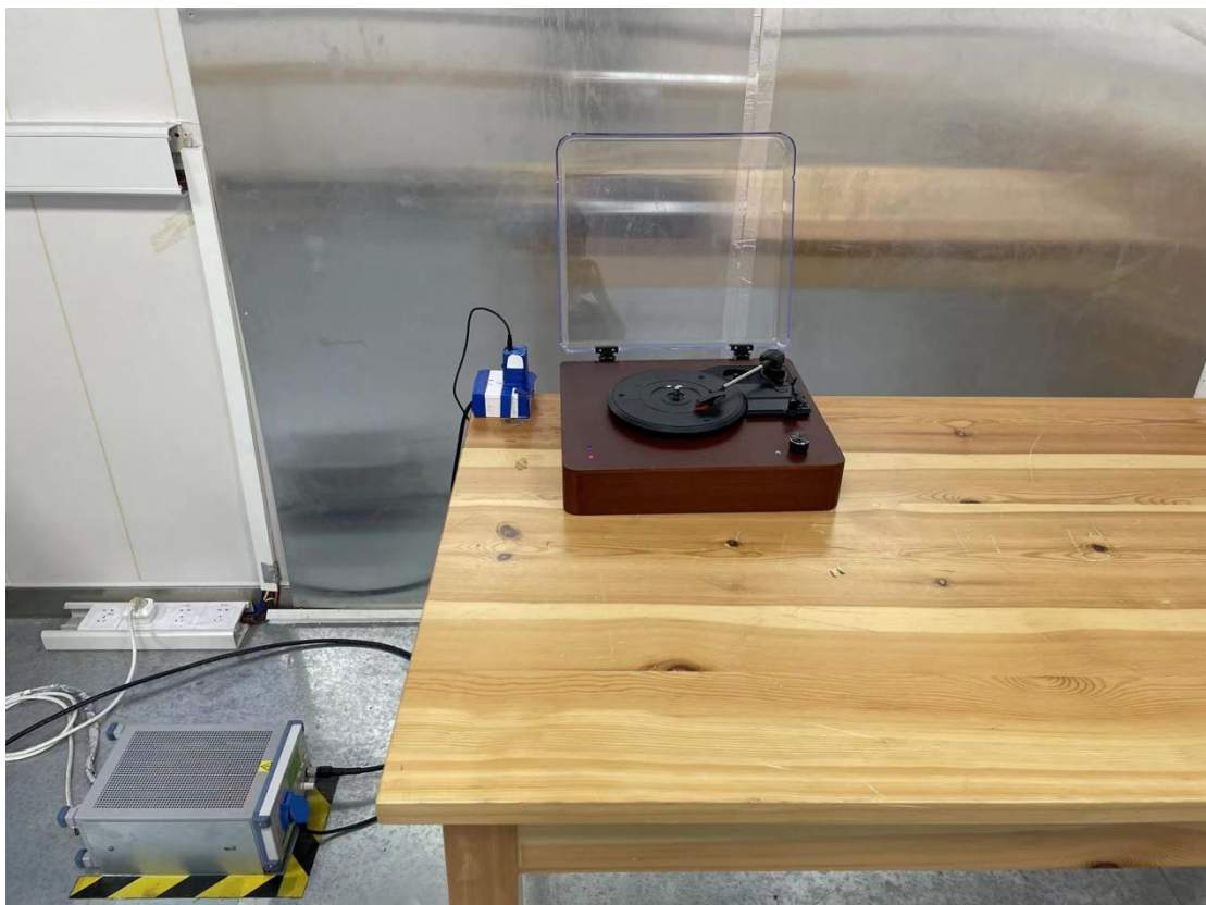
Conducted emission test setup
