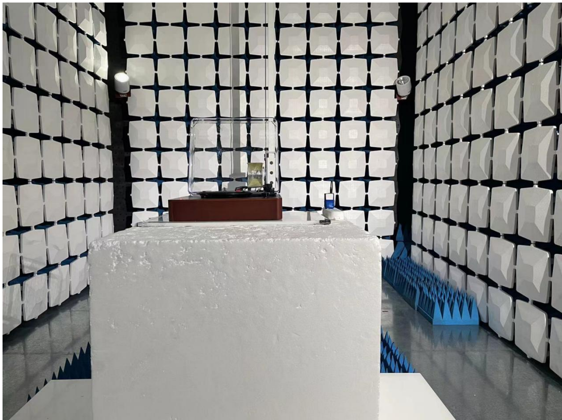
Above 1GHz for radiated emission test setup
