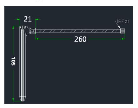
Product physical 2.4G-5.8G dual frequency white ultrasonic antenna 1.13 gray wire output length 260MM
