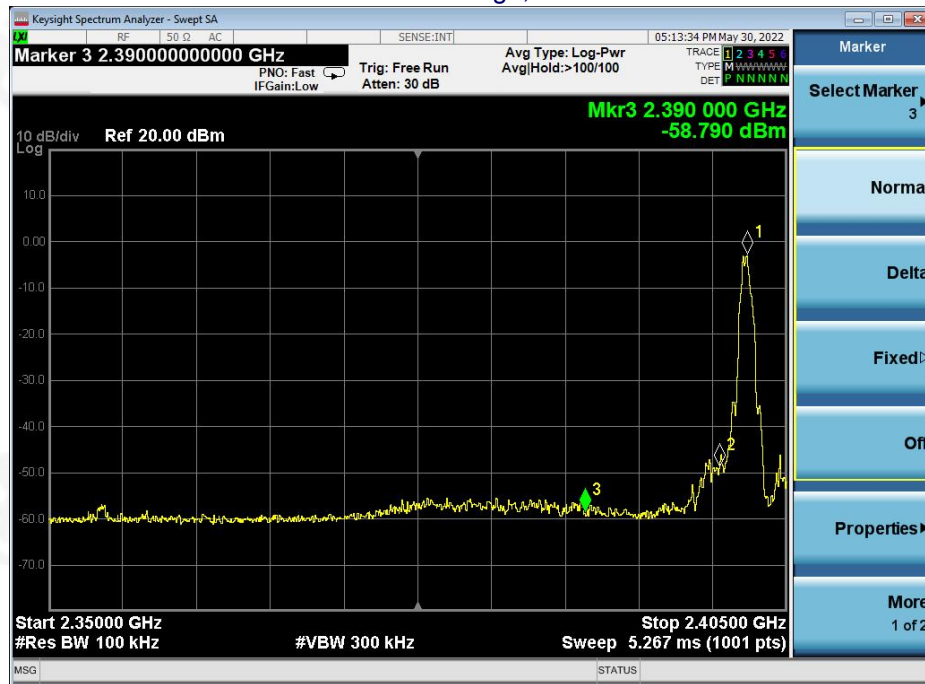
GFSK: Band Edge, Left Side
