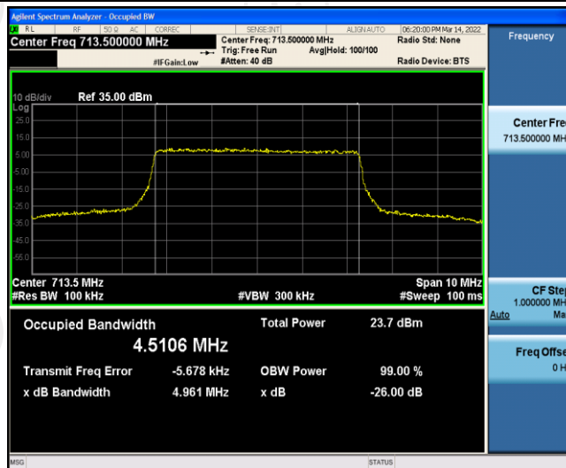
Band17-10MHz-QPSK-23780-50RB#0
