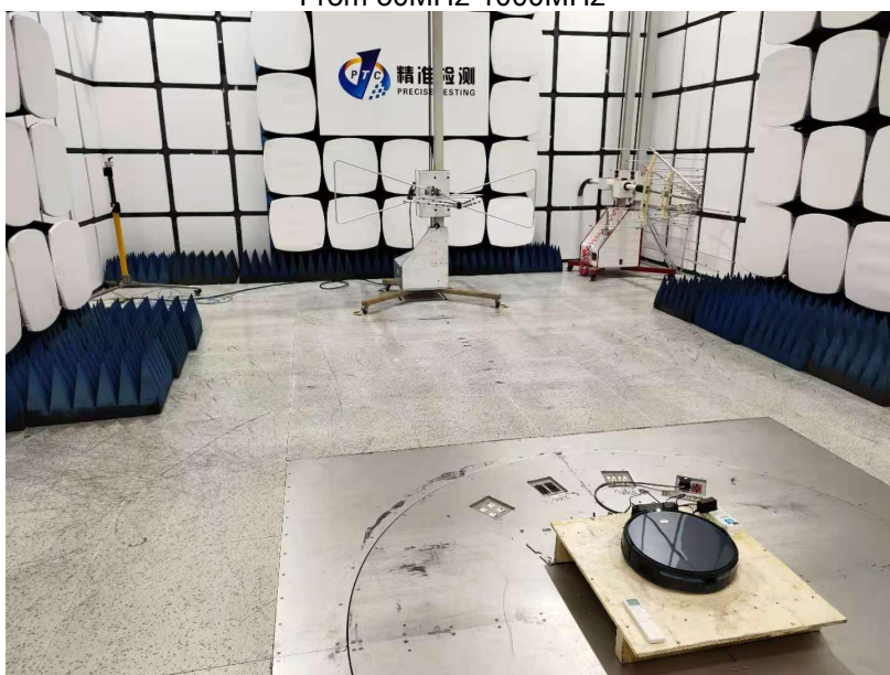
Radiated Spurious Emissions From 30MHz-1000MHz
