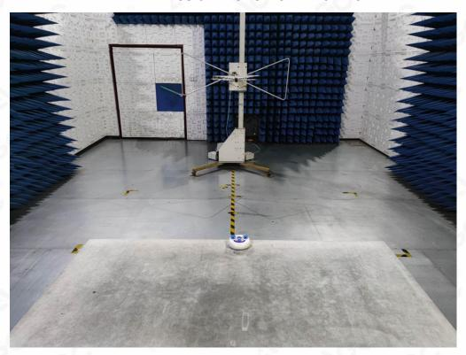
RADIATED EMISSION TEST SETUP ABOVE 1GHz
