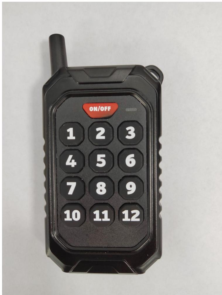
ON/OFF: 1. Control the total on/off of the load
