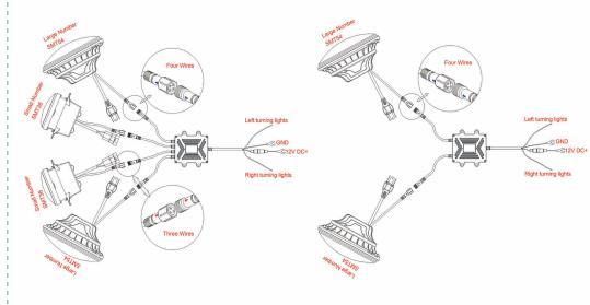
one by four(two pc headlight,two pc fog lamp)
