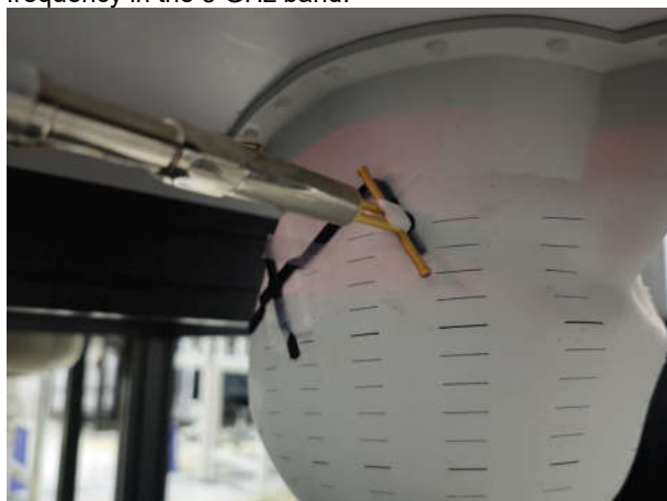
2.4GHz Dipole Placed at Location C in 90° Orientation (10mm Spacer)
